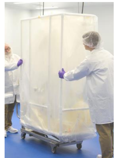
FIGURE 5.1: ABEC single-use bioreactor bag, packaged for sterilization and shipping [211].
